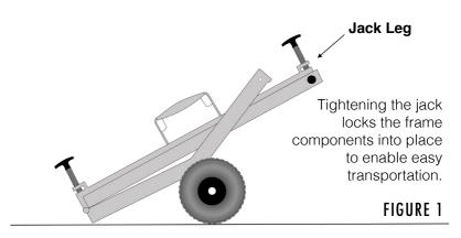
Release jack leg, pull and lift the handle which will separate the bearer beam from the 'Load' handle.
